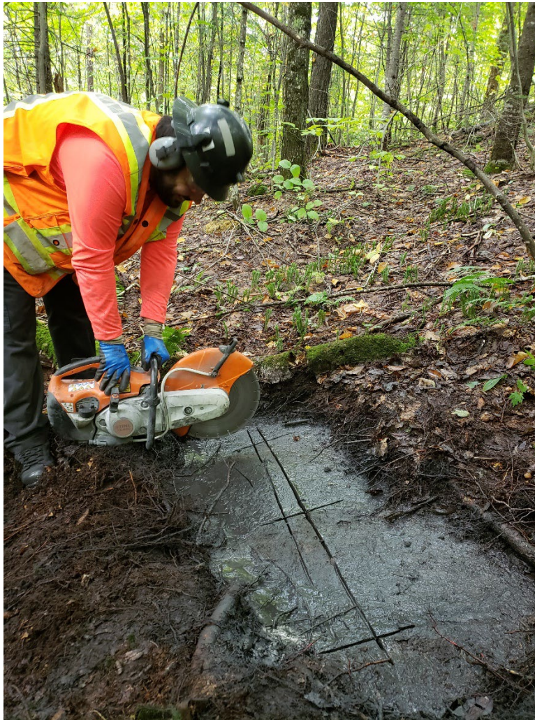
Figure 12 – GMG’s technician operating the rock saw to collect channel samples on VLF-40.
