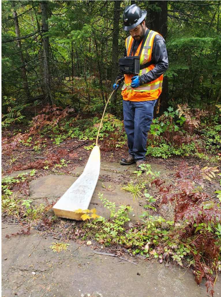
Figure 11 – The Beep-Mat Electromagnetic survey on exposed outcrops at the Property.
