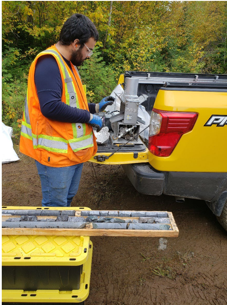
Figure 17 – GMG’s technician uses the hydraulic core splitter to split the core into two halves.
